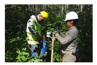
Student researchers from the University of Alberta install state-of-the-art wireless sensor networks in remote forests around the world to monitor high resolution photosynthesis and seasonal productivity trends to help track patterns in carbon dynamics near the Earth's surface. Photograph by: Cassidy Rankine
